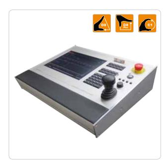
The I-Motion Basic-C controller, which belongs to the Basic controller family, constitutes a compact system controller for the systemic control of kinetic drives in mobile and flexible project applications.
