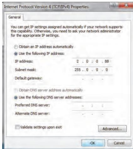
7 Open the SGM Rail Light Configuration Tool, select the appropriate ethernet interface, and click 'OK'
