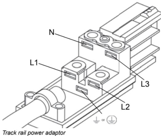
The fixture must be grounded/earthed and be able to be isolated from AC power. The AC power supply must incorporate a fuse or circuit breaker for fault protection.
